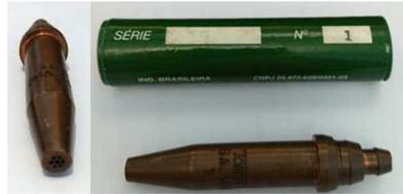
Figure 3 – Cutting tip Torch 3502 series number 1.
