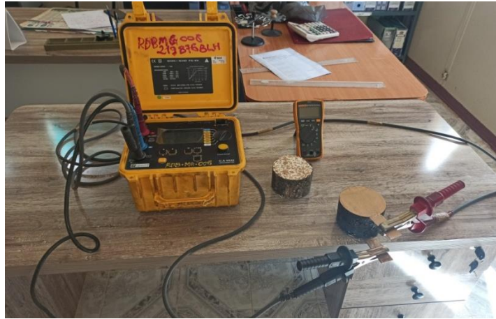
Figure 6 – Measures electrical resistance using the two-point method.
