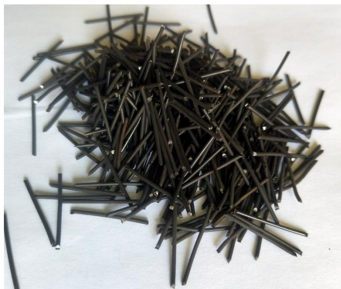
Figure 1 - Waste steel tiers fibers recycled from tiers
