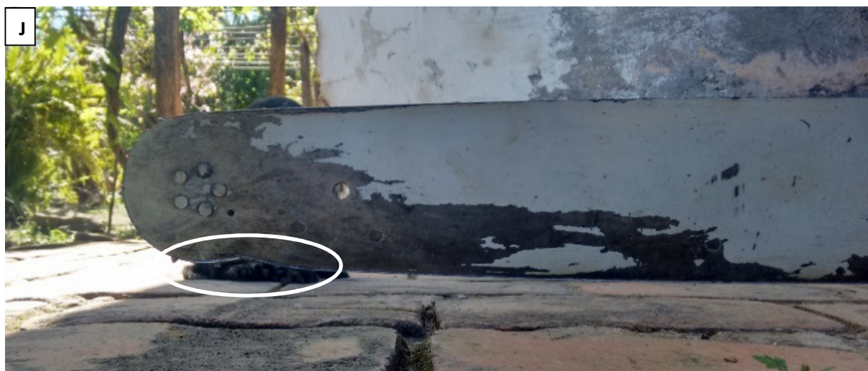
Figure 1. Conservation conditions of chainsaws regarding general maintenance (A, B, C, D); chainsaw without manual chain break and front hand guard (E); lack of chain catcher pin (F); lack of safety throttle (G); air filter needing a cleaning (H, I); worn saber (J)
