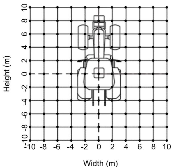
**Figure 1.** Sample grid of the levels of noise produced by the backhoe. The dark dots are the sample points
