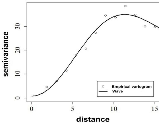
**Figure 2.** Semi variogram of the noise produced by the backhoe
