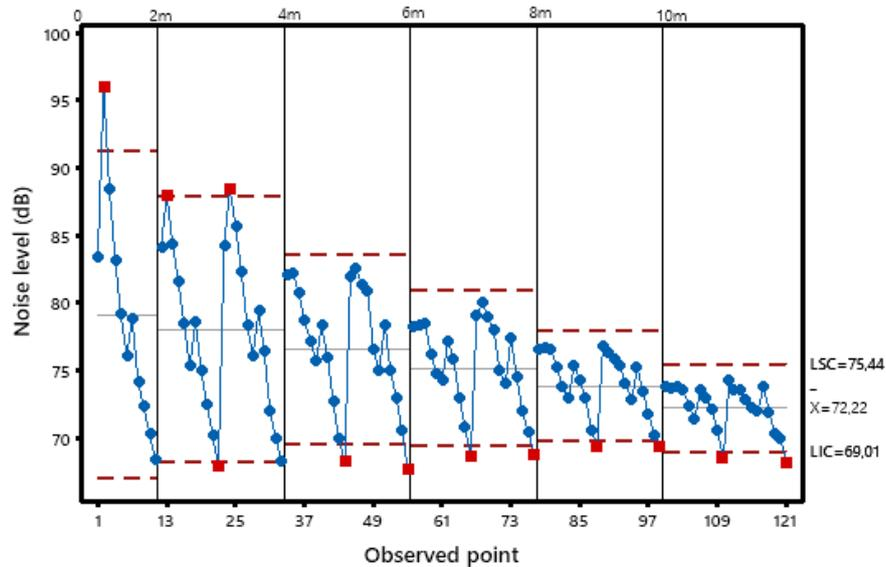
**Figure 6.** Control chart for the noise levels of the backhoe
