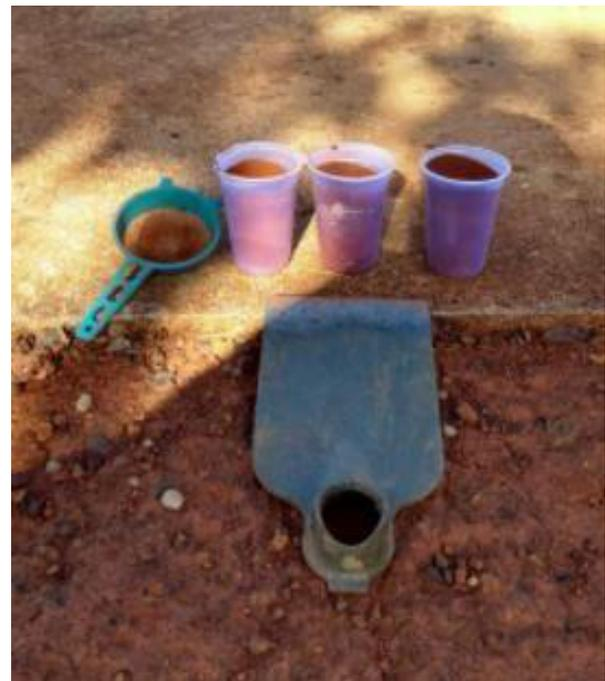
**Figure 3.** Soil sample collection for capacitive sensor calibration
