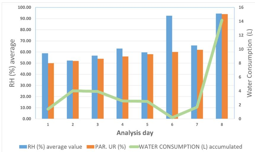
**Figure 11.** Relation of relative air humidity and water consumption
