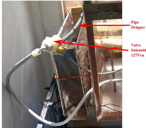
**Figure 2.** Air humidifier-radiator hydraulic system
