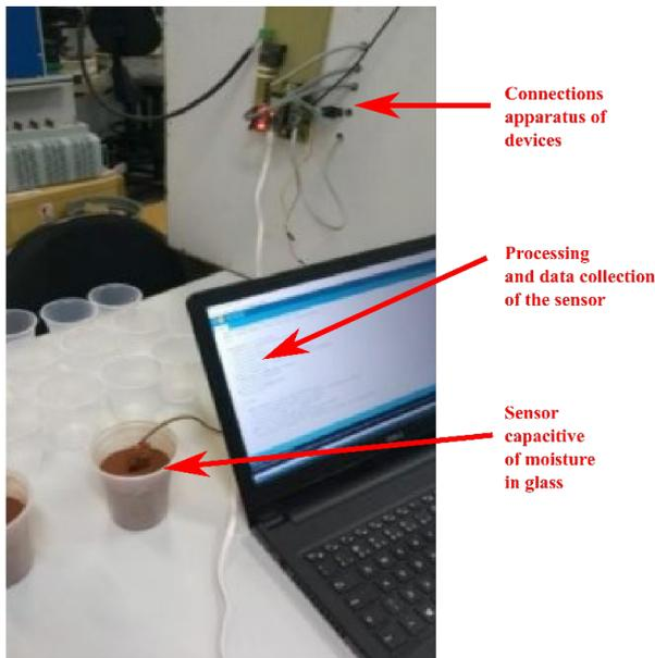
**Figure 5.** Start of capacitive sensor calibration
