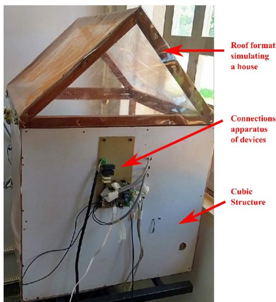
**Figure 1.** View of the greenhouse structure
