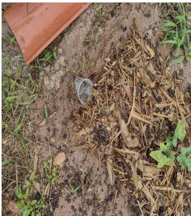
**Figure 7.** Plastic container for collecting surface runoff, installed at the lower end of the experimental plot, at ground level and following a 45° slope
