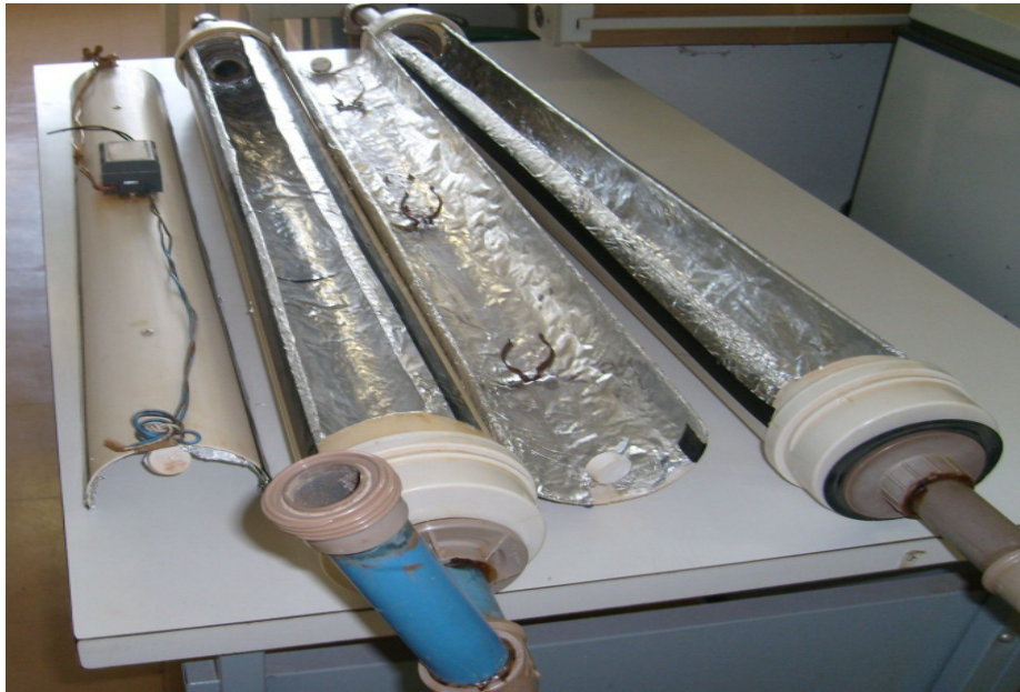
Figure 2. Photo-reactors coated with aluminum foil.
