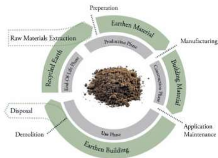
Figure 3 – Earthen building materials and methods - Life cycle diagram of earth as a building material.
